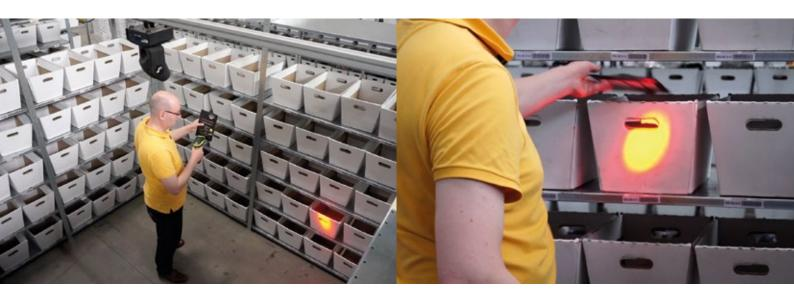
Through the intelligent use of proven technology we have developed an innovative solution for light-guided pick and put processes. In contrast to conventional systems, the shelf is not fitted with lighting equipment; instead, a spot of light is projected onto the targeted object.
